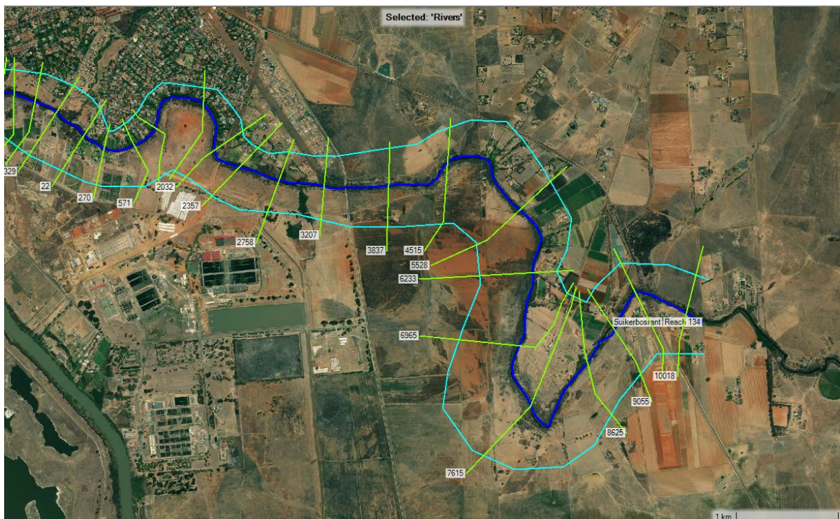
Figure 6-1: Modelled river section geometry used in the simulation of the floodlines
